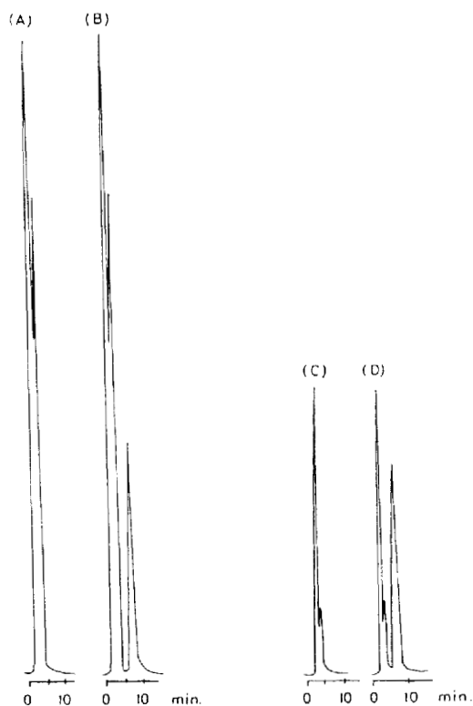
Figure 5. Chromatograms: (A) Blank urine. (B) Urine containing 10.0 \mu\text{g/ml} MGBG. (C) Blank serum. (D) Serum containing 1.0 \mu\text{g/ml} MGBG. Separation was carried out on octadecylsilane bonded-phase column. Mobile phase containing 0.05 M phosphate buffer pH = 3.0, methanol (80:20) and 1.0 mM sodium heptane sulfonate. Flow-rate : 1.0 ml/min.
